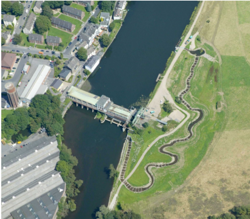
Figure 3.12: Nature-like bypass channel Harkortsee hydropower station, Ruhr River, Germany (Photo: Ruhrverband)
