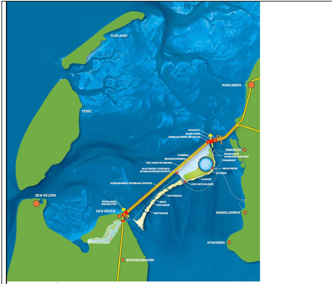
Figure 5.8: Renovation plans of the Afsluitdijk including the construction of a energy storage “Valmeer” according to the Natuurlijk Afsluitdijk consortium.
