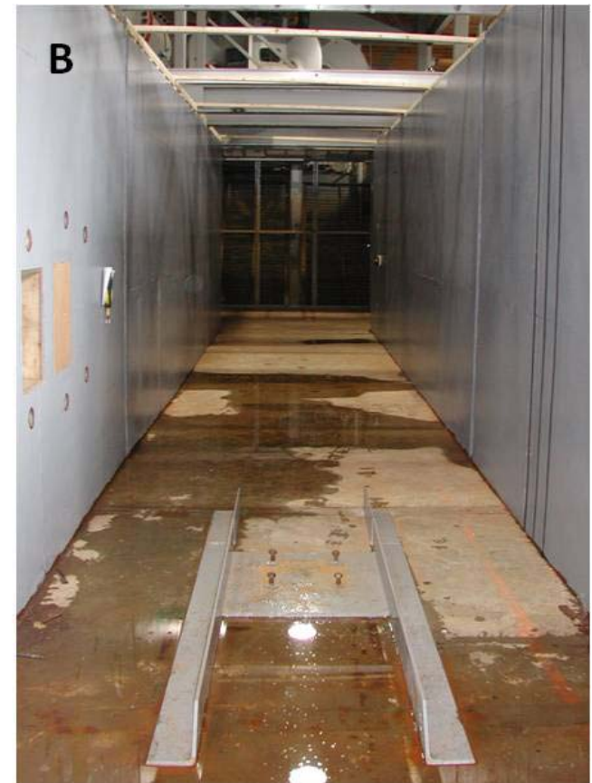
Figure 2-6 Downstream View (A) and Upstream View (B) of Alden's large flume fish testing facility configured for the biological evaluation of hydrokinetic turbines with constricting walls installed
