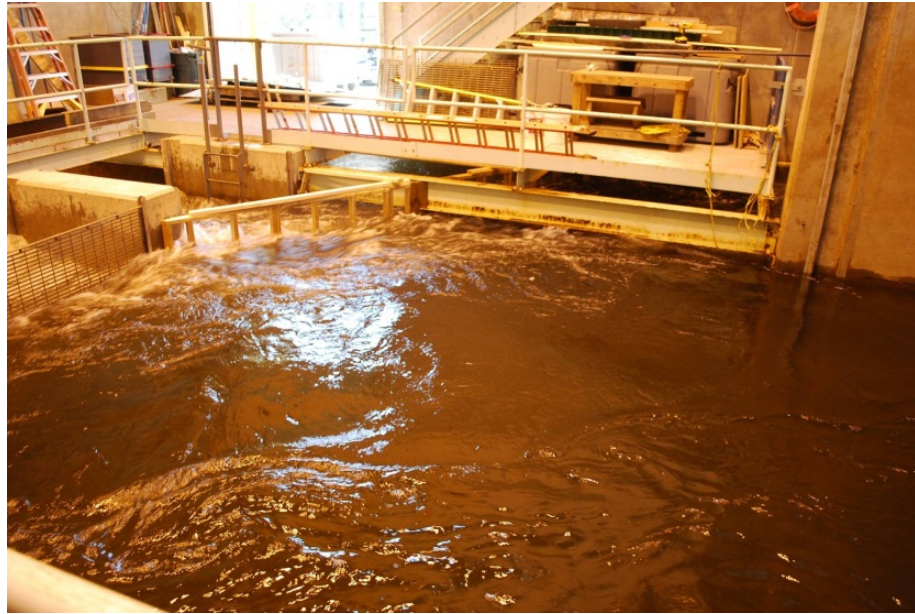
Figure 2-4 Downstream staging and recovery area. Discharge is toward the left; test flume is out of sight in background, behind the concrete wall to the right. The screen continues to arc toward the back wall as shown in Figure 2-1. Note the slack water condition, which provided suitable resting conditions for both Atlantic salmon and American shad.
