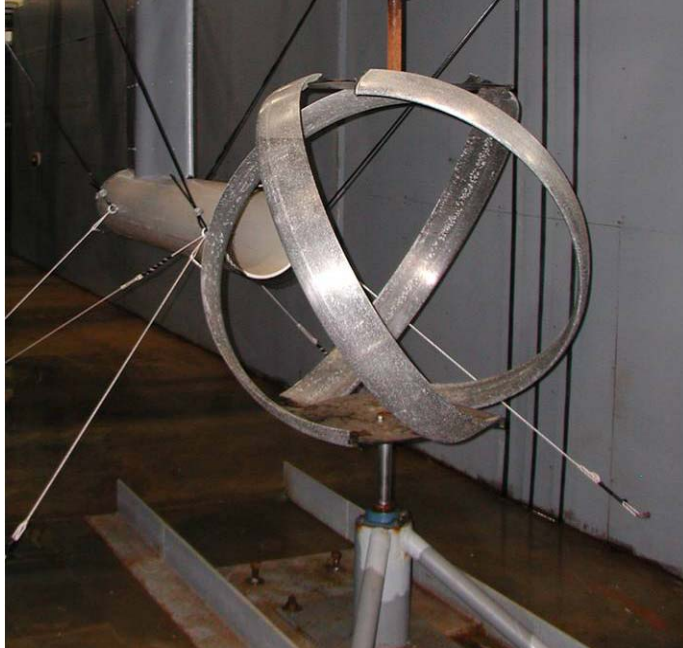
Figure 2-1 Lucid spherical turbine installed in Alden's test flume for fish testing
