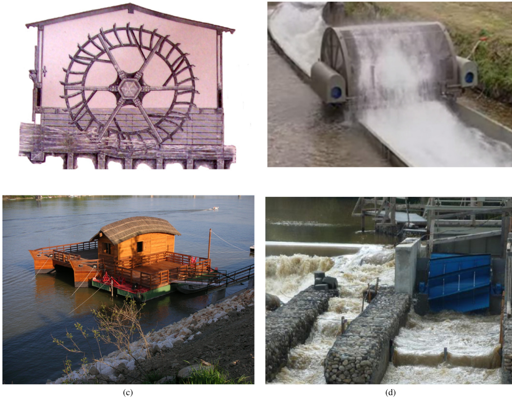
Fig. 3. Stream water wheels in: (a) subcritical shallow flow (Quaranta, 2017), (b) supercritical shallow flow (photo of Emanuele Quaranta), deep flow (photo courtesy of AIAMS Italy) (c), and Hydrostatic Pressure Machine (picture of Nick Linton) (Linton, 2013) with diagonal blades to reduce drag at the blades (d).
