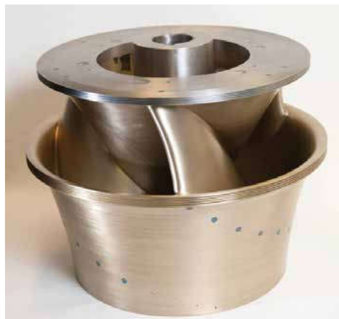
Figure 2. Alden turbine physical model (1:8.7 scale) used for performance testing by Voith Hydro. Photo credit: Alden Research Laboratory.
