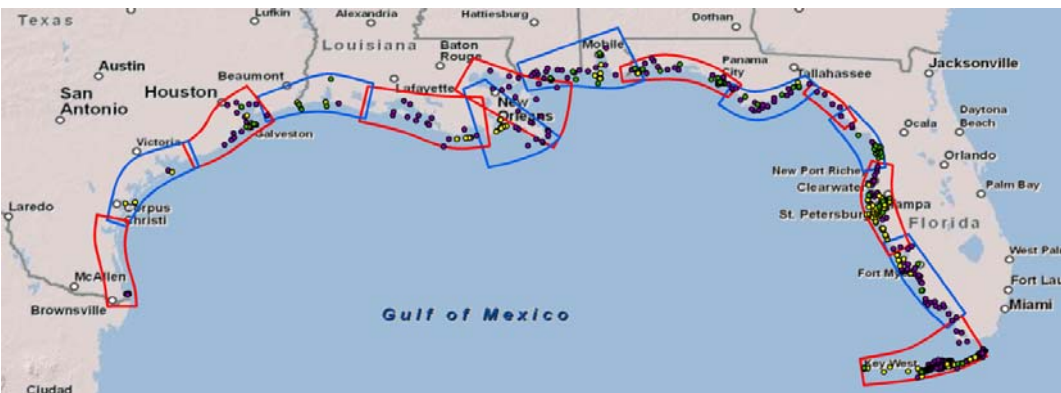
Figure 4. Map of computational grids and the calibration data sources. Harmonic constituents for tidal currents (green) and water levels (black), and prediction for maximum current (yellow) and high/low tide elevations (purple).
