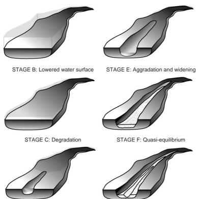
Fig. 1. Conceptual model of channel changes through time in reservoir following removal of a small dam (adapted from Doyle et al., 2003a).
