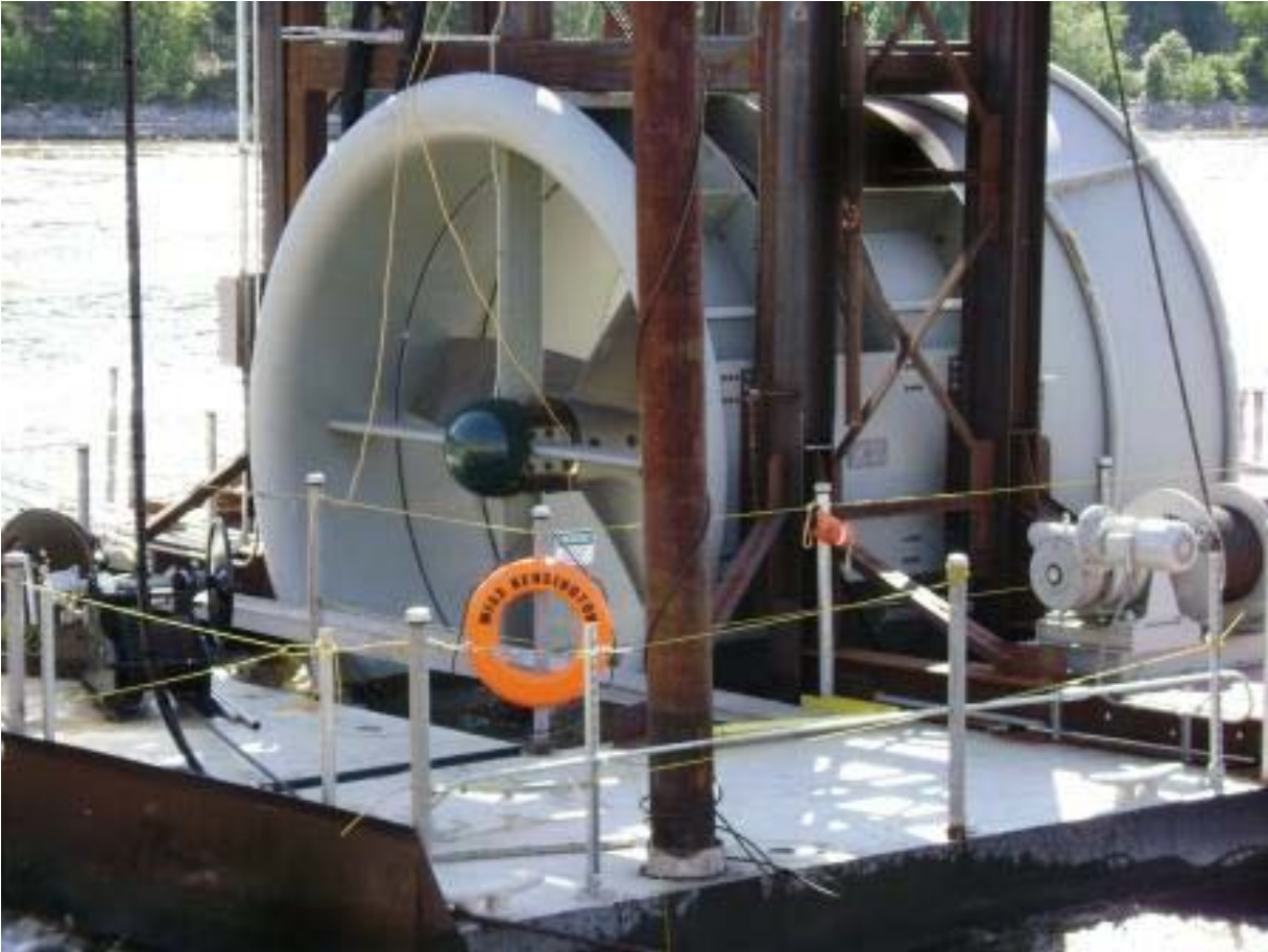
Figure 1-3. HGE hydrokinetic turbine prior to submergence in the tailrace of the Mississippi Lock and Dam No. 2 Hydroelectric Project near Hastings, MN.
