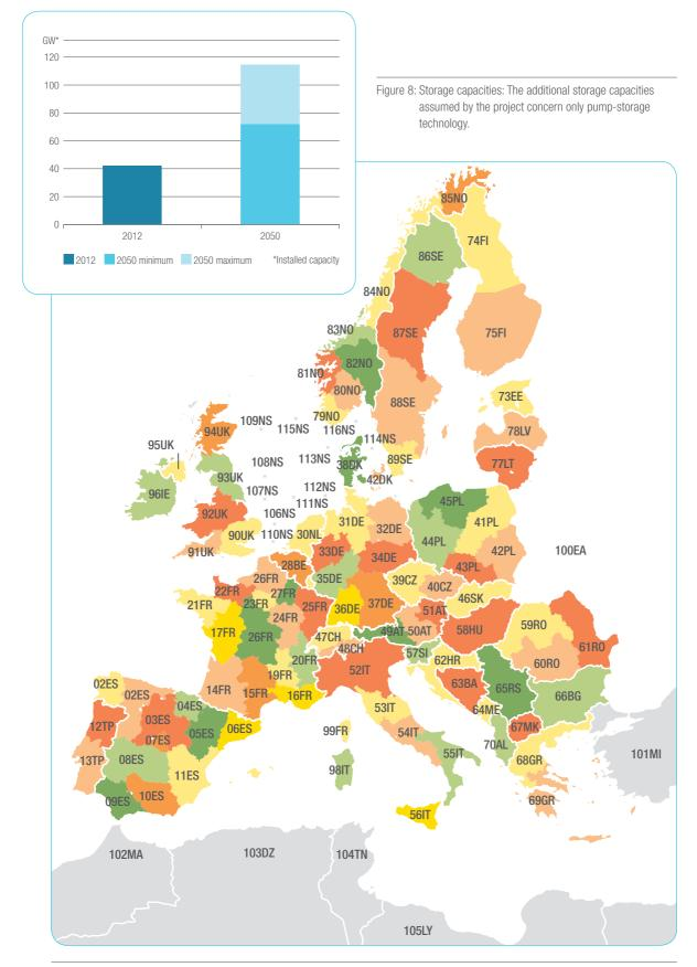
Figure 7: Model with 100 clusters: For the study, the European power system is represented via a zonal model with 100 clusters. Demand and installed capacities for each generation technology have been defined per cluster, and for each scenario. © EuroGeographics for the administrative boundaries
