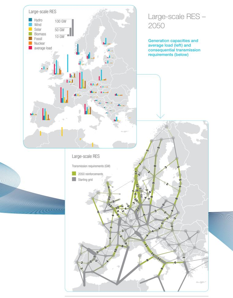
Figure 12 E: Transmission requirements identified in scenario Large-scale RES (GW)
