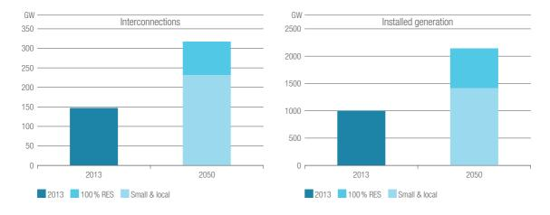
Figure 15: Interconnection capacities: The left figure presents the cumulative interconnection capacities (physical and not commercial). The increase foreseen by 2050 is consistent with the evolution of the installed generation.
