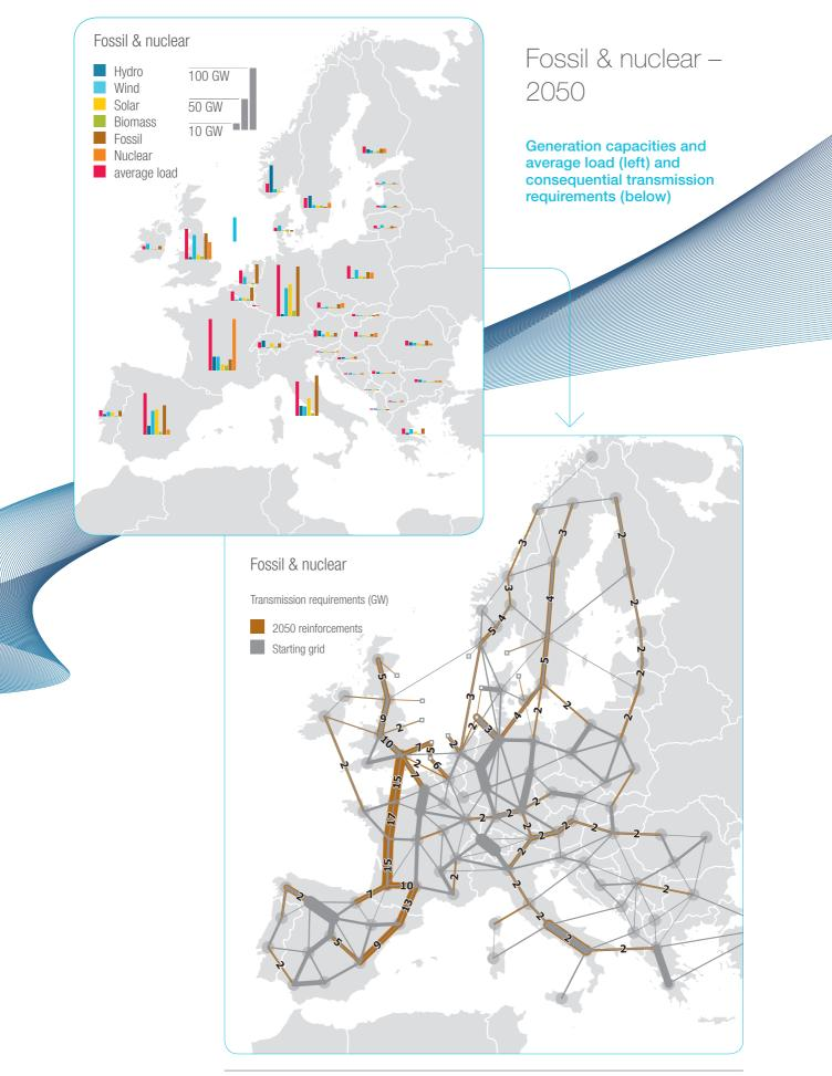
Figure 12 C: Transmission requirements identified in scenario Fossil & nuclear (GW)
