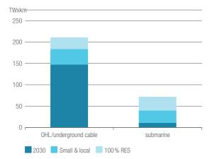
Figure 13: Transmission infrastructure capacities: The indicator shows the cumulative transmission grid capacities in TWxkm present in 2030, and the proposals for two extreme scenarios in 2050. This indicator includes new and refurbished infrastructures. In total, the increase is between + 40 % and 90 %, equally split between land and submarine.
