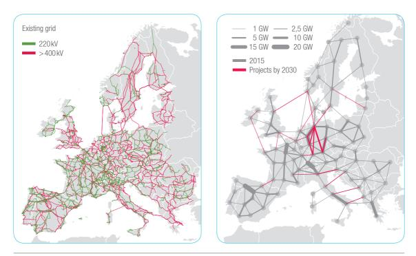
Figure 9: Starting grid of the e-Highway2050 project. Existing grid (left) and equivalent model of the 2030 grid (right, the grey lines represent the existing lines and the red ones represent the projects to be realised by 2030 at the point in time of starting the simulations).
