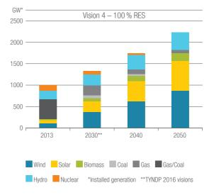
Figure 6: Trajectories of the European installed generation per technology from 2013 to 2050 for three e-Highway2050 scenarios
