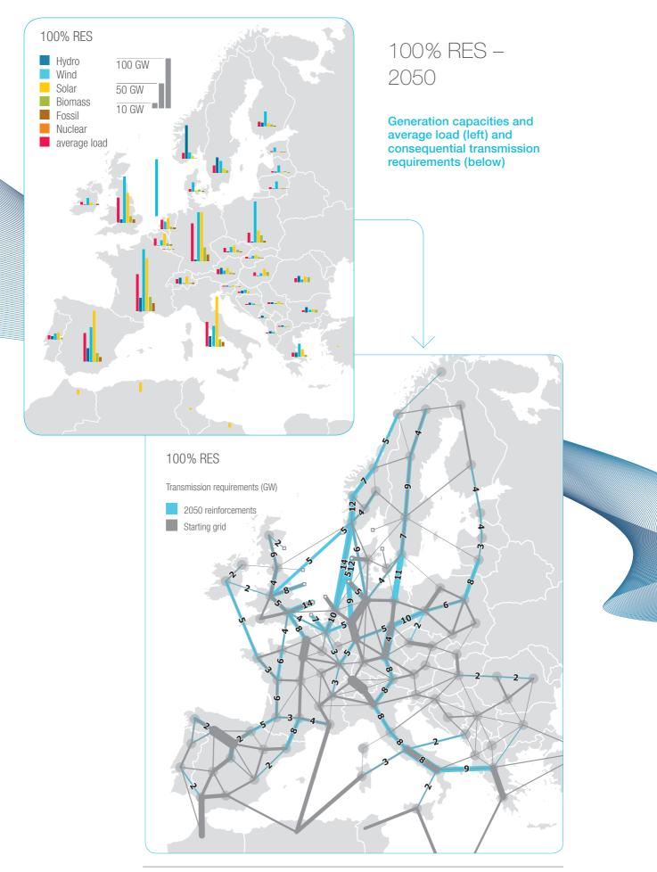
Figure 12 D: Transmission requirements identified in scenario 100 % RES (GW)
