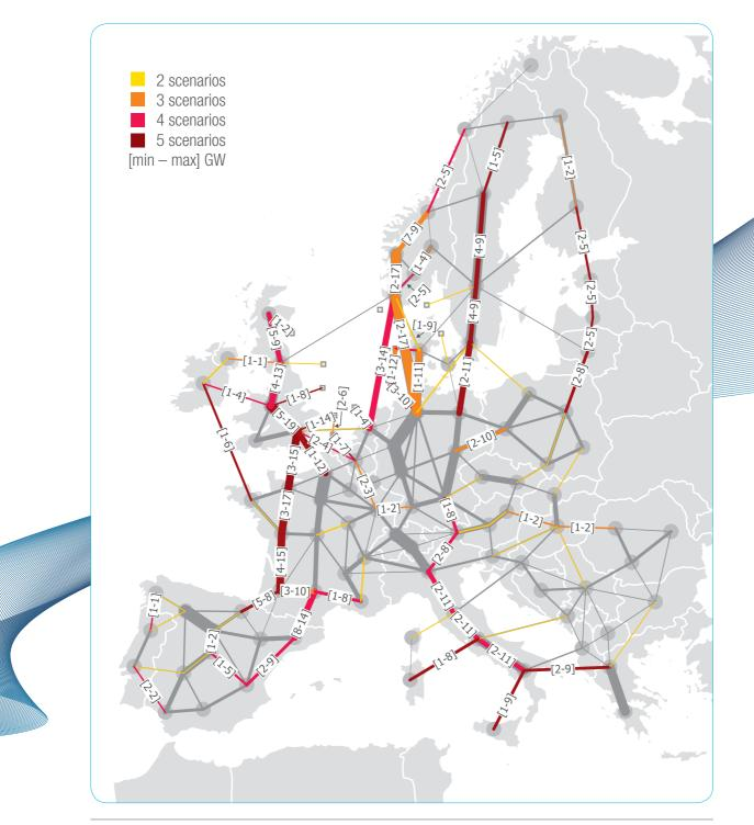
Figure 14: Common reinforcements (widths are according to average reinforcement capacity and the colour represents the number of scenarios where the reinforcement is needed)
