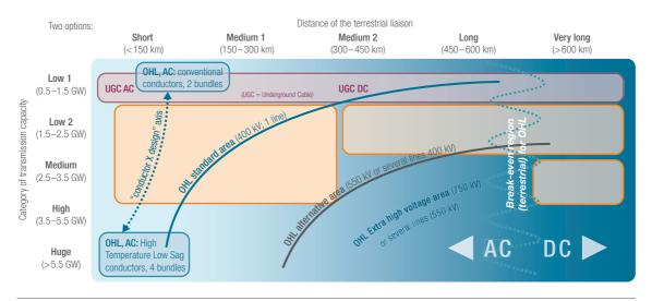
Figure 19: RD&D gap analysis: terrestrial needs (orange cells) compared to available technology options (OHL options: various grades of blue, from the more conventional to the less conventional; terrestrial cables options: in purple color)
