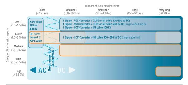
Figure 20: RD&D gap analysis: submarine needs identified in the simulations (orange cells) compared to available technology options (blue cells)
