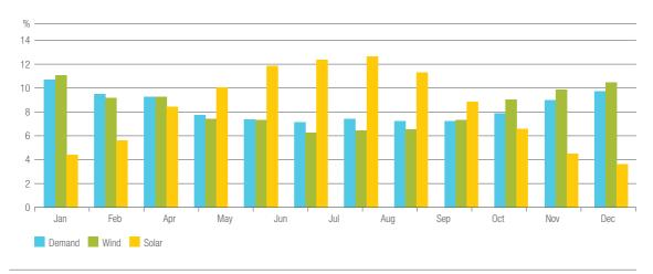
Figure 24: Monthly distribution of the solar and wind generations, and of the demand
