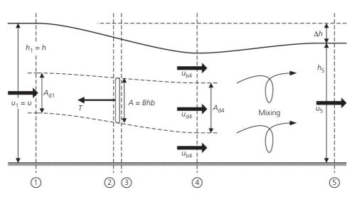
Figure 1. One-dimensional LMADT in an open channel flow
