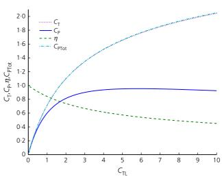
**Figure 7.**  $C_{TL}$  against  $C_T$  (dotted),  $C_P$  (solid),  $\eta$  (dashed) and  $C_{PTot}$  (dot-dashed) for B = 0.20, Fr = 0.20
