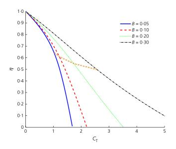
**Figure 3.**  $C_{\rm T}$  against  $\eta$  for four blockage ratios: B = 0.05 (solid), B = 0.10 (dashed), B = 0.20 (dotted), B = 0.30 (dash-dotted). Fr = 0.20 for all cases.  $\eta$  at peak  $C_{\rm P}$  is plotted with the double dashed line
