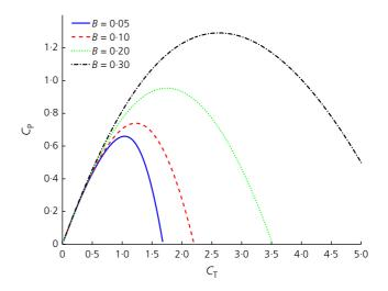
**Figure 2.**  $C_{T}$  against  $C_{P}$  for four blockage ratios: B = 0.05 (solid), B = 0.10 (dashed), B = 0.20 (dotted), B = 0.30 (dash-dotted). Fr = 0.20 for all cases
