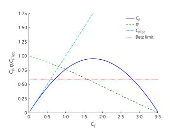
**Figure 6.**  $C_{\rm T}$  against  $C_{\rm P}$  (solid),  $\eta$  (dashed) and  $C_{\rm PTot}$  (dot-dashed) for B = 0.20, Fr = 0.20. The Betz (1920) limit is illustrated with a dotted line
