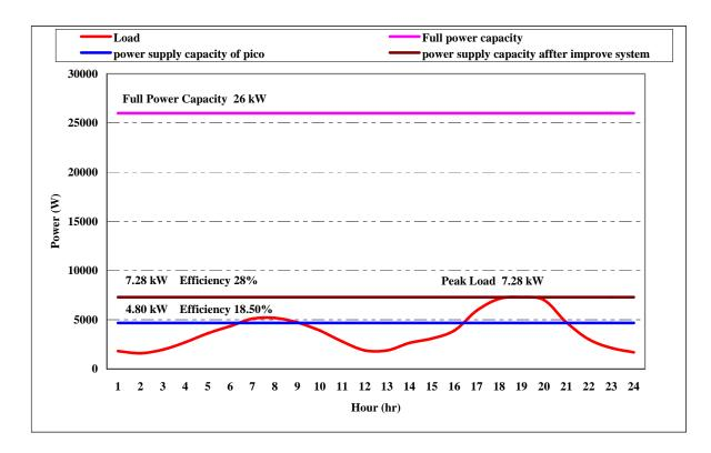
Fig. 7 Load Profile after improve the Efficiency Demand peak load 7.28 kW Power Supply Capacity 7.28 kW Out put Supply Efficiency 28 % Number of family 50 Household Load demand per family 145 W
