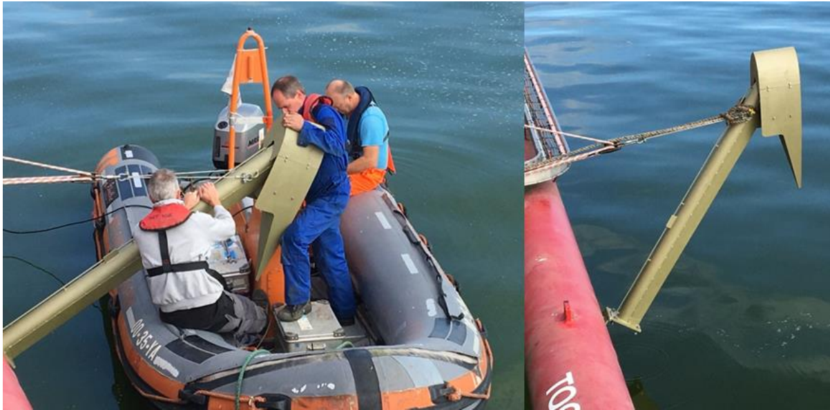
Figure 7.4. Mounting the lift cable/ropes to the streamlined waterbody housing the DIDSON (left) so that the housing device can be fixated in a uplift position above the water (right).
