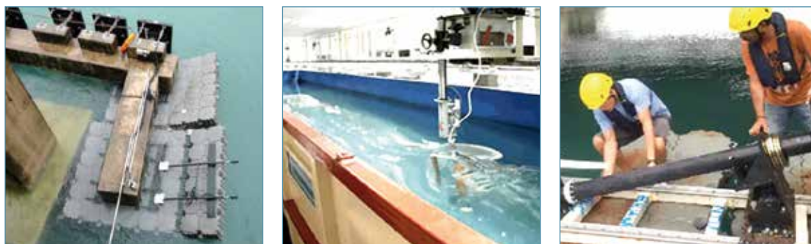
Floating hinged turbine support frame to house tidal turbines and vortex induced vibration devices (Left), Scaled (1:3) tidal turbine in tow tank (Middle) and successful deployment of the turbine at Sentosa Test site. (Right)
