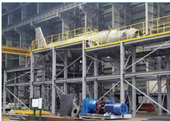
200 kW active-controlled tidal energy converter in fabrication and installation of its substructure
