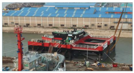
300 kW Floating pendulum wave energy converter in port
