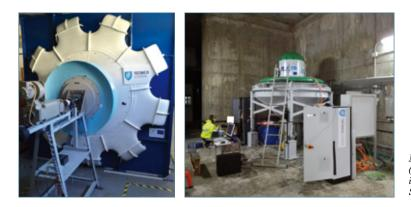
Model testing of the twin-rotor air turbine (left) at IST; biradial turbine prototype installed at the OWC-breakwater, Mutriku, Spain (right).
