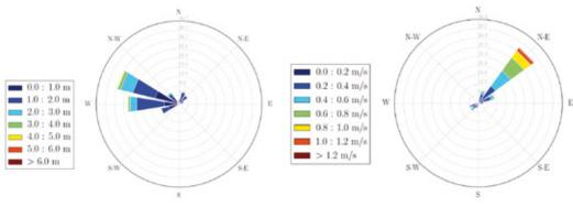
Directional measurements of waves and currents at the DanWEC Hanstholm site
