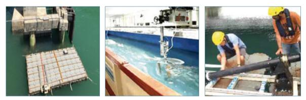
Floating hinged turbine support frame to house tidal turbine devices(Left), Scaled (1:3) tidal turbine in tow tank (Middle) and successful deployment of the turbine at Sentosa Test site. (Right)
