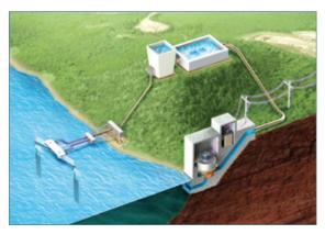
${\cal A}$  schematic of the tidal current and pumped storage hybrid power generation system
