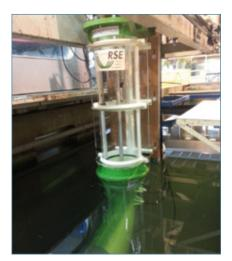
The WAVESAX 1:5 scale prototype
