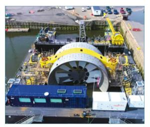
Cape Sharp Tidal's 2 MW turbine in port after successful recovery.
