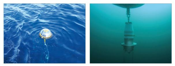
ZUNIBAL oceanographic buoy (left) and DITREL subsea connector (right) tested at BIMEP.
