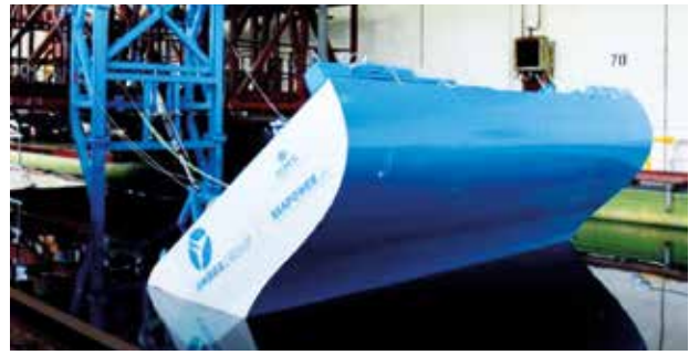
The PIVOT full-scale prototype (5 m width), in the wave tank of University of Naples "Federico II"
