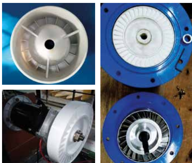
Unidirectional turbine / Bidirectional turbine
