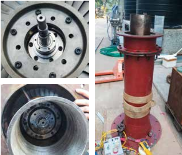
Open Cycle OTEC turbine for laboratory studies
