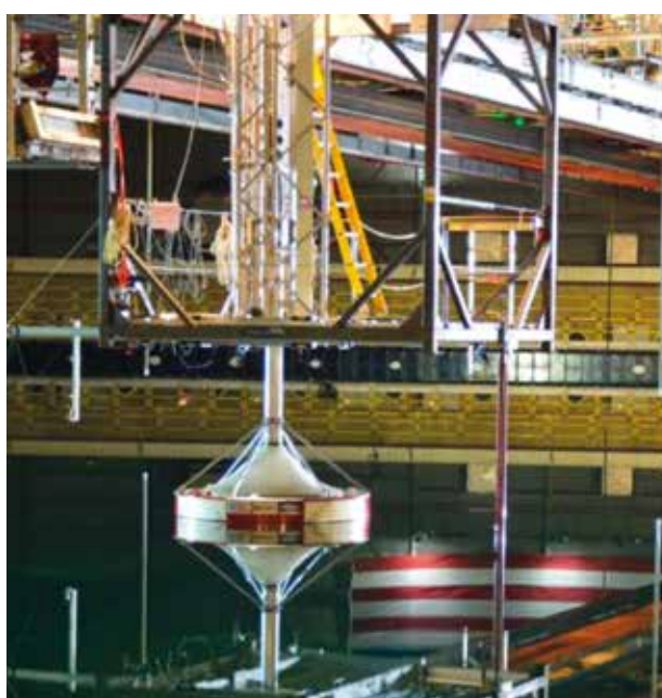
Heaving, surface piercing wave energy concept tested at the US Navy MASK and used as a test case for numerical modelling validation
