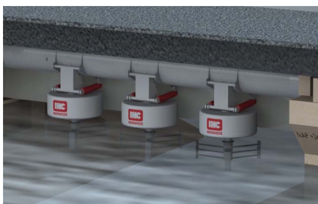
Figure 8.2 Reactive (ducted) Free Stream Configuration, Left example project Waterdunen (Tocardo), Right Oosterschelde surge barrier (IHC)
