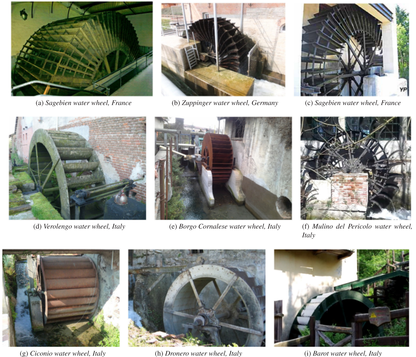
Fig. 4. Water wheels in operation. The top figures are undershot water wheels, the figures at the center are breastshot water wheels, while the figures at the bottom are overshot water wheels. Representative dimensions of some water wheels are reported in Table 5. Photo courtesy of: (a) Patrick H. Marceau, (b) Prof. Müller Gerald, (c) Marie-Paule Dupuy, (d) (g) (h) research project ORME conducted by the Authors, (e) (f) Quaranta Emanuele, (i) mulino Moriena di Fenile di Campiglione, Michel Moriena.
