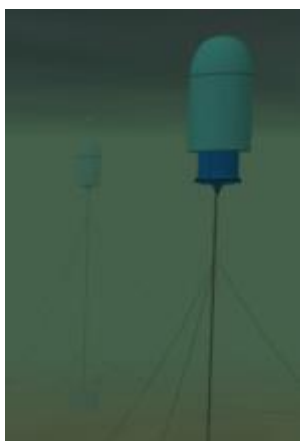
Figure 23 Symphony looks like the Archimedes Wave Swing, but houses an innovative linear power take off system using an air pressure chamber and sliding bellow frames.
