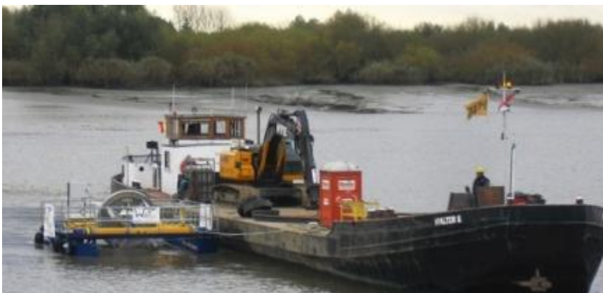
Figure 14 Water2Energy being towed in the Scheldt river near Temse for testing as part of the Pro-Tide R&D project.
