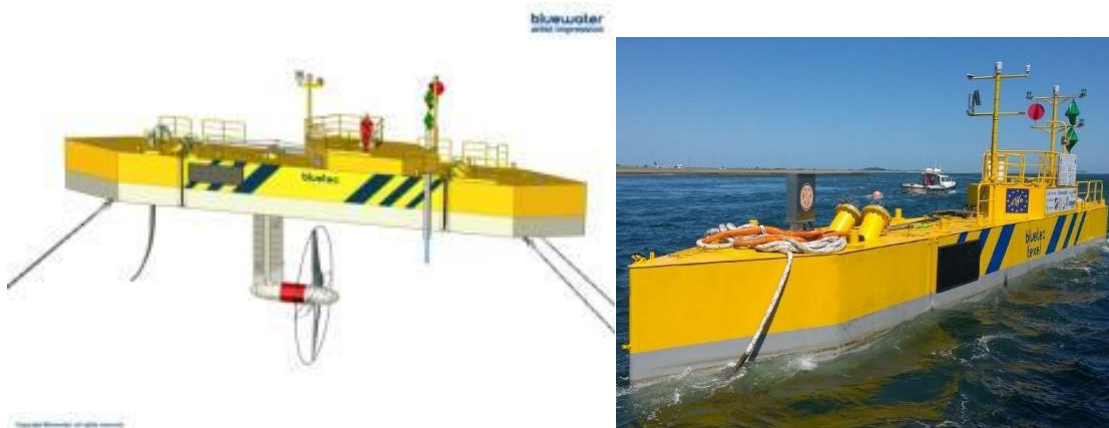
Figure 16 Single turbine floater (200kW) for autonomous power supply for coastal communities recently installed at the Tidal Testing Centre offshore pilot zone near Texel.
