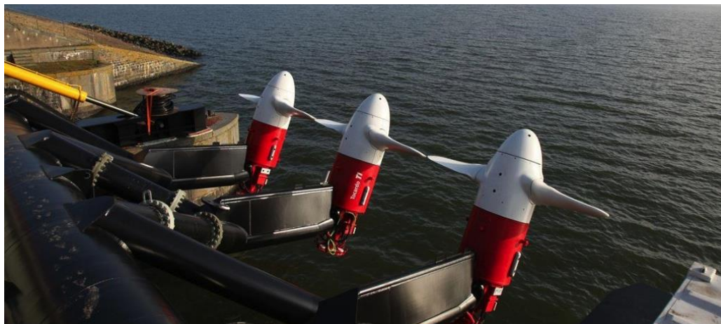
Figure 7 Tocardo T1 turbine during push tests in the Wadden Sea in 2013, Tocardo T1 turbine mounted under the BlueTEC platform before installation in the Marsdiep and an array of three Tocardo turbines in the Afsluitdijk
