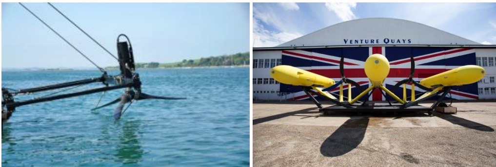
Figure 9 Left: Schottel 3m turbine being tested at the test site of Queen University Belfast in Strangford Lough, Northern Ireland, Right: two Schottel turbines mounted on the Plat-O platform before deployment in the Solent (near Isle of Wight, UK)
