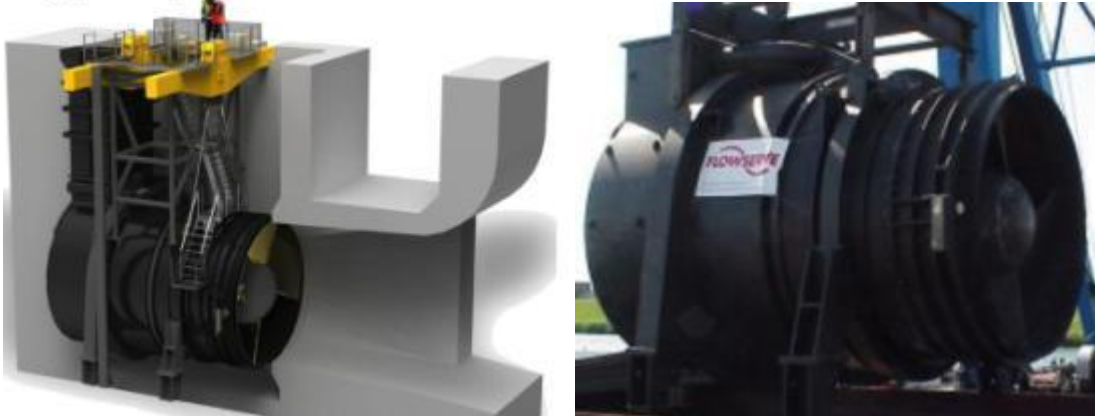
Figure 13 Left: Flowserve bulb turbine design, right: typical Flowserve pump
